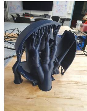
Figure 2: Iteration 0: organic FDM prototype, used to validate the servo-bearing-wheel stack geometry.
